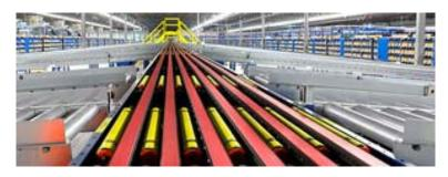
TGW's narrow belt sorter conveyor is specifically designed for quiet operation, but also reduces operating costs, energy consumption and maintenance. The belts, running in a track instead of one wide belt, produce a smooth product flow while maximizing your sort rate. Additionally, this type of conveyor endures a long belt life.
